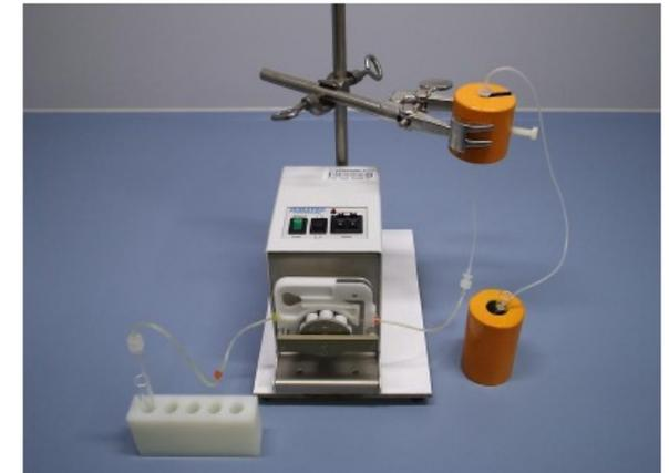
Ac-225/Bi-213 generator in lead shielding with peristaltic pump for semiautomatic elution
